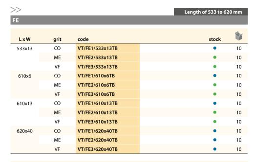
The FE-grade is mainly used for short belts. These are used for applications where the edge durability is the most important.
